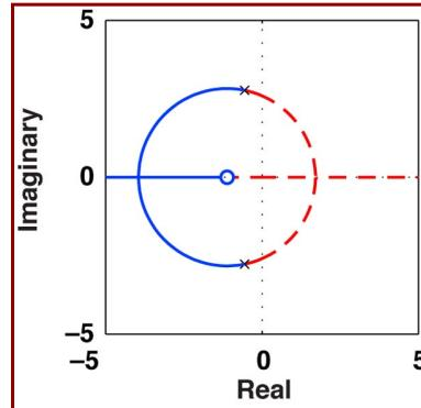
$$\Delta(s) = \left\{ s - \left[ \frac{L_\alpha}{2V_N} + \sqrt{\left( \frac{L_\alpha}{2V_N} \right)^2 + M_\alpha} \right] \right\} \left\{ s - \left[ \frac{L_\alpha}{2V_N} - \sqrt{\left( \frac{L_\alpha}{2V_N} \right)^2 + M_\alpha} \right] \right\} - k \left( s + \frac{L_\alpha}{V_N} \right) = 0$$
