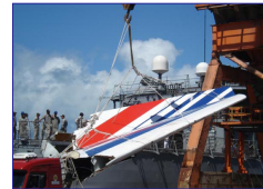
"Visual examination showed that the airplane was not destroyed in flight; it appears to have struck the surface of the sea in level flight with high vertical acceleration."
